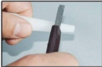
1. Cut off the extra part of the extension nozzle
